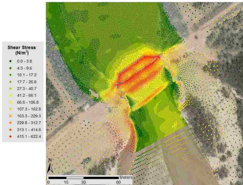
Figure 89: SRH-2D shear stress results at 226.5 m 3 /s modeled discharge
