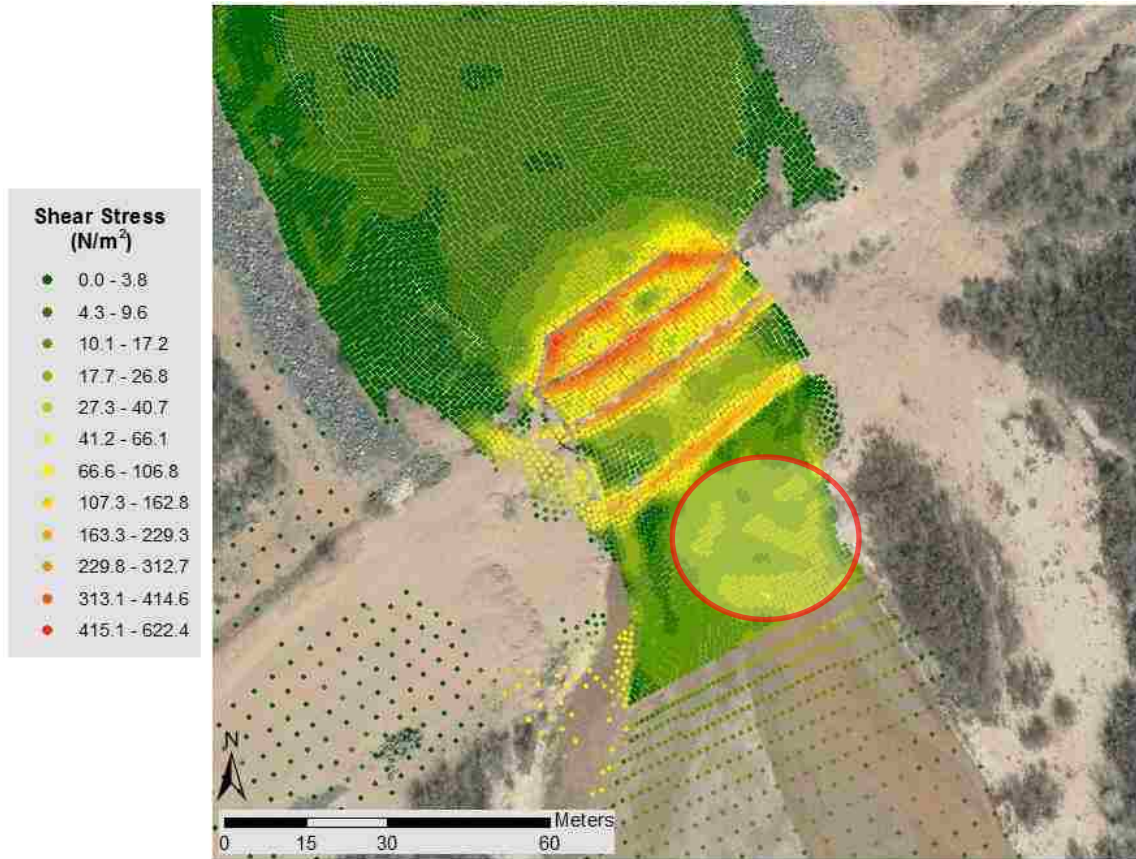
Figure 26: Shear stress results near the Jemez Weir for 28.3 m 3 /s modeled discharge
