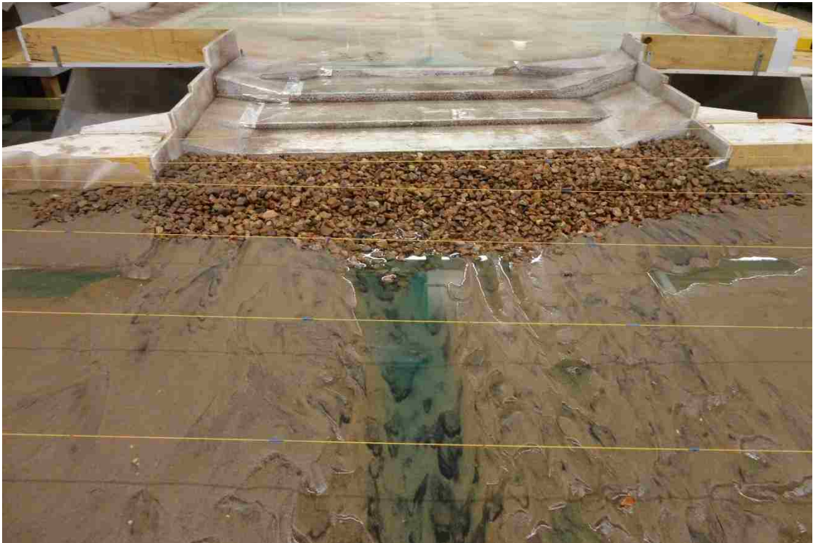
Figure 7: Counter measure with additional large rock and starting bed elevation 1580.8 m (post modeling)
